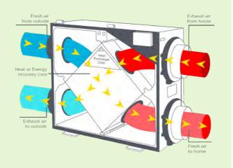
ERVs do have associated energy costs for the fan energy, however they recover substantial more energy than is consumed. – Typically HRVs recovery around 80% of energy in the exhaust stream. Further, the necessary capacity of the mechanical conditioning system is reduced when combined with an ERV.
