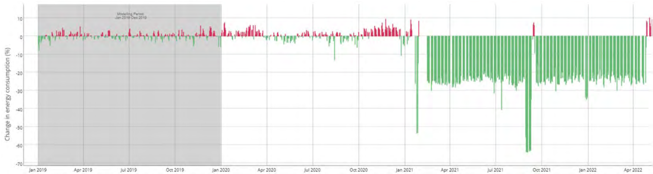
Figure 12 CCHR electricity metering 2019 to 2022 showing data anomaly due to incorrect meter wiring
