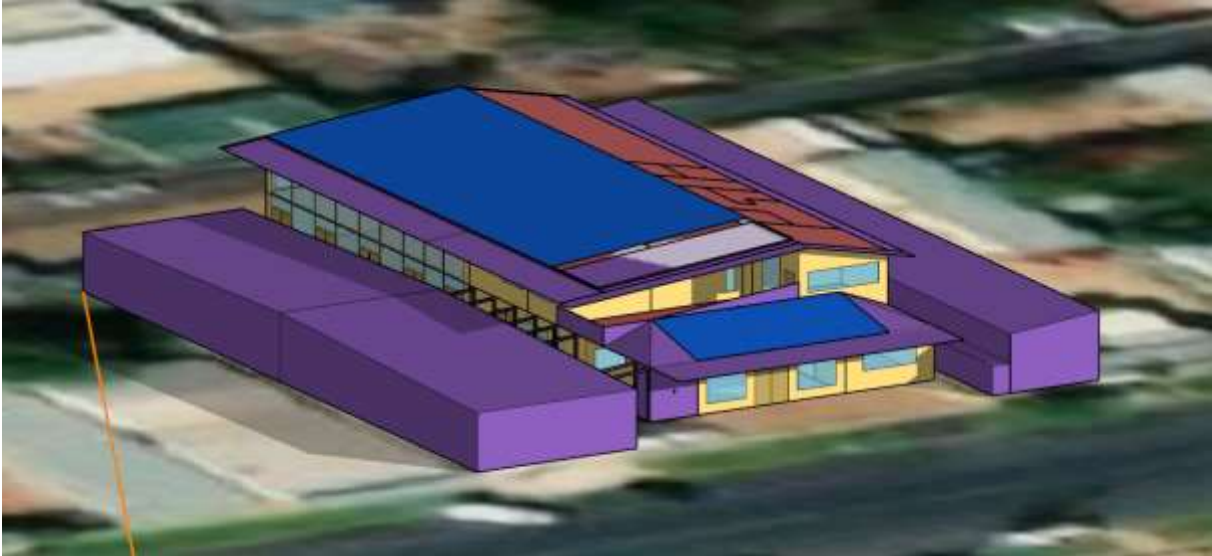
Figure 5.3.2: Proposed Secondary solar location on LALC building
