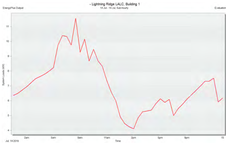
Figure 5. 14 th of July peak Heating load
