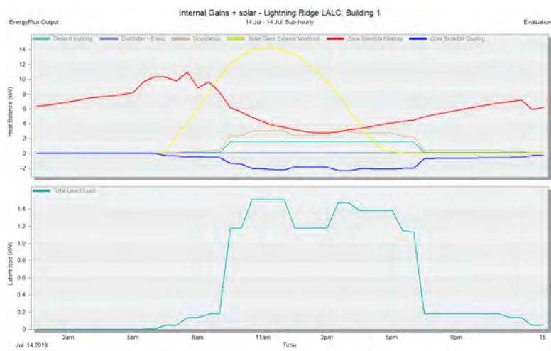
Figure 7. Internal gains and solar on the 14 th of July
