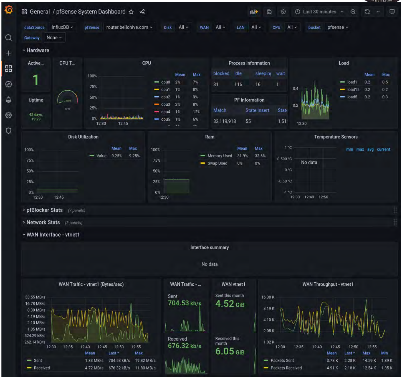
Figure 30: InfluxDB - Grafana dashboard, connected to the same InfluxDB instance, rendering pfSense router data
