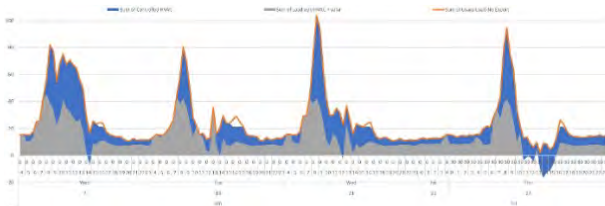
Figure 129: preliminary finance - CCP3 Jamison HS select days in June and July where HVAC controls is affecting load
