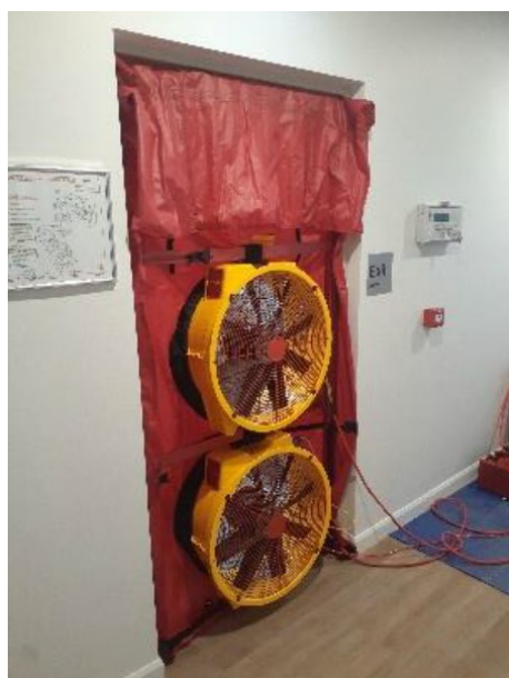
Figure 3-14 Blower door locations
