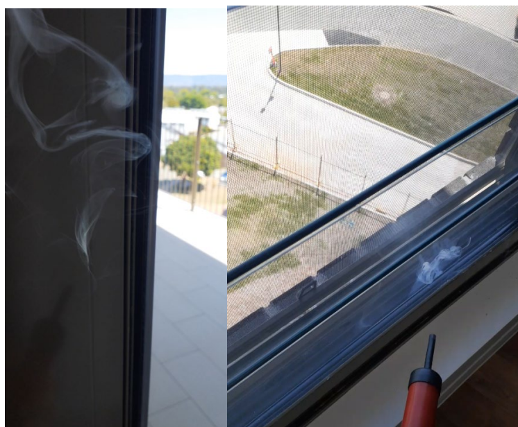
Figure 3-16 Air leakage path in windows
