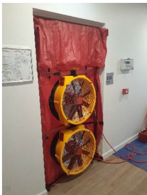
Figure 3-14 Blower door locations
