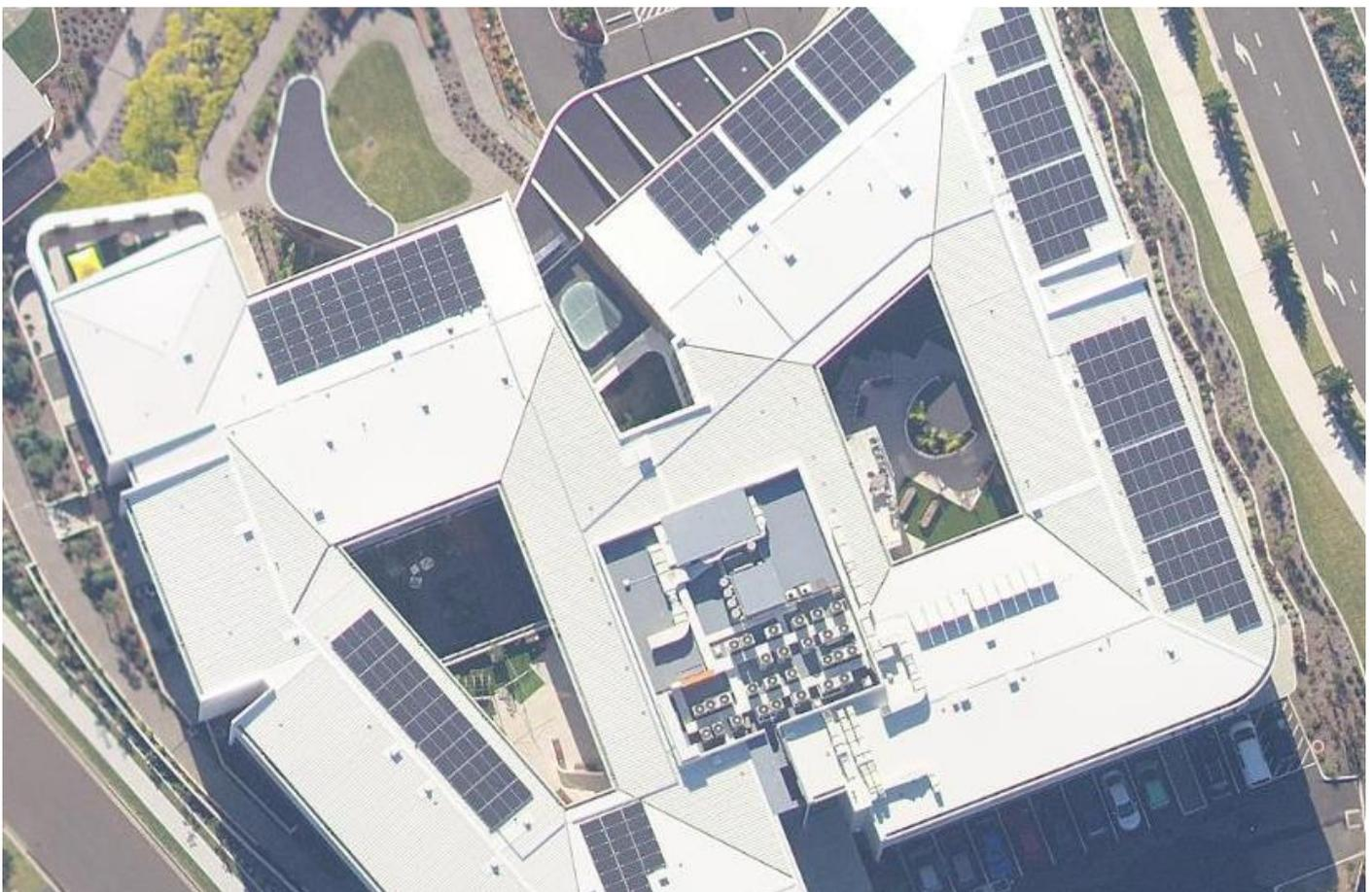
*Figure 5 - Aerial view of the living laboratory with the 99 kWp PV system and HVAC service on the roof.*
