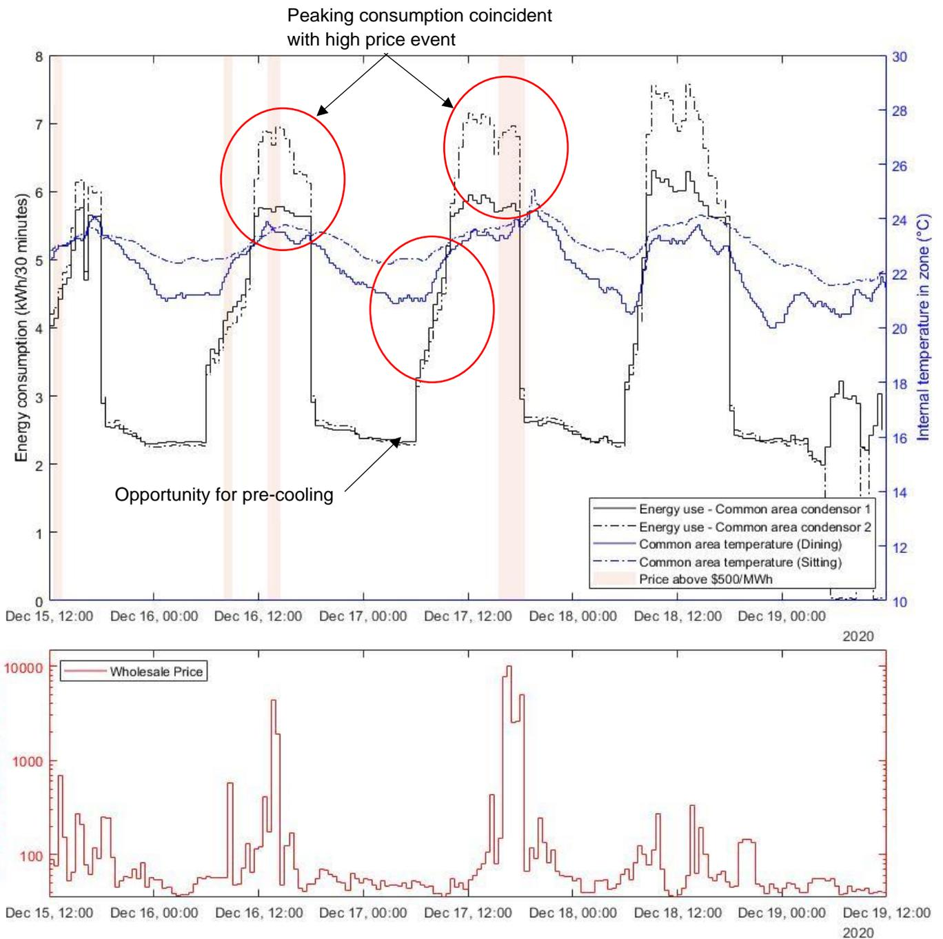
Figure 7. Summer time-series measured data from the Warrigal living laboratory showing energy use for individual condenser units, co-incident internal temperatures for a sample of the zones serviced by these units, and co-incident wholesale spot price during a period with a number of high price events.
