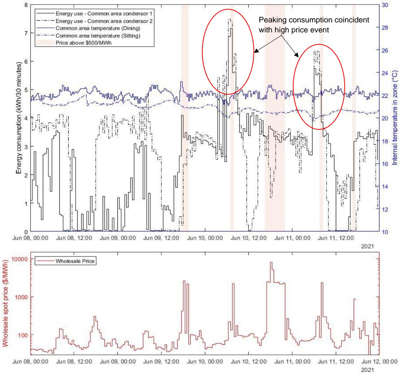
Figure 8. Winter time-series measured data from the Warrigal living laboratory showing energy use for individual condenser units, co-incident internal temperatures for a sample of the zones serviced by these units, and co-incident wholesale spot price during a period with a number of high price events.
