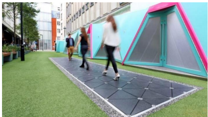
Piezoelectric walking mats, image sourced by Haziq Azul Rahmam, Uni Melbourne
