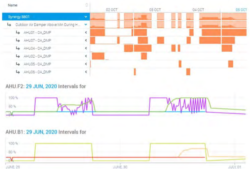
Figure 12: Indicating excessive outdoor air
