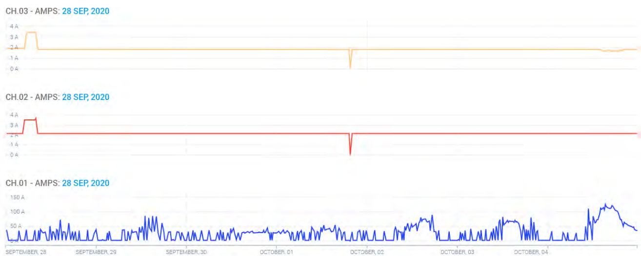
Figure 10: Indicating excessive and incorrect chiller cycling
