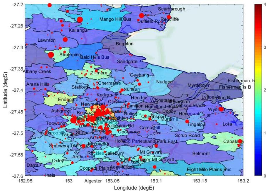
Figure 3 Demand response available from commercial building HVAC in Greater Brisbane, as a mean percentage of sub-station load during peak times (area shading). Dots indicate concentrations of commercial buildings.
