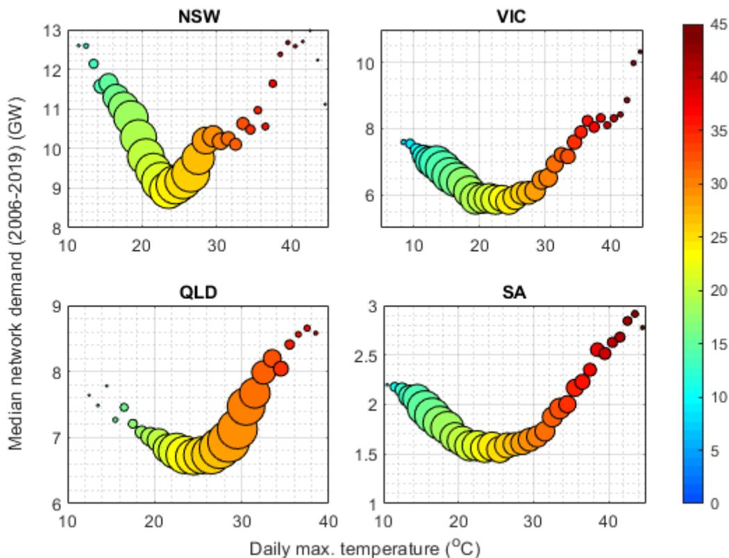
Figure 1 Median network demand as a function of temperature by NEM state (marker size indicates time duration).
